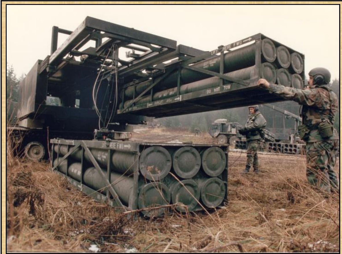
Figure 3-f Reload Operation: Launcher crew members perform a reloading operation using the built in boom and hoist assembly of the M269 Launcher Loader Module (LLM). The LLM turret has two bays, with each being capable of handling a two and a half ton Launcher Pod/Container (LP/C). From the time the SPL launcher stops, to the time it moves off, the launcher will have only taken ten to twenty minutes to reload five tones of ordnance. (Photo courtesy of, Lockheed Martin, Missiles and Fire Control.)
