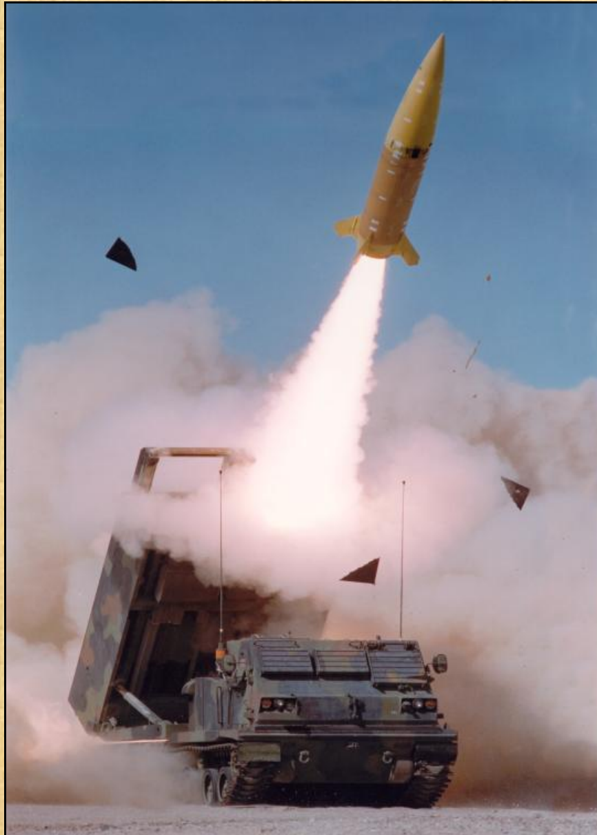
Figure 3-j Missile Launch: A test launch of the M39 ATACMS at White Sands, New Mexico pictured in the first moments after ignition.
