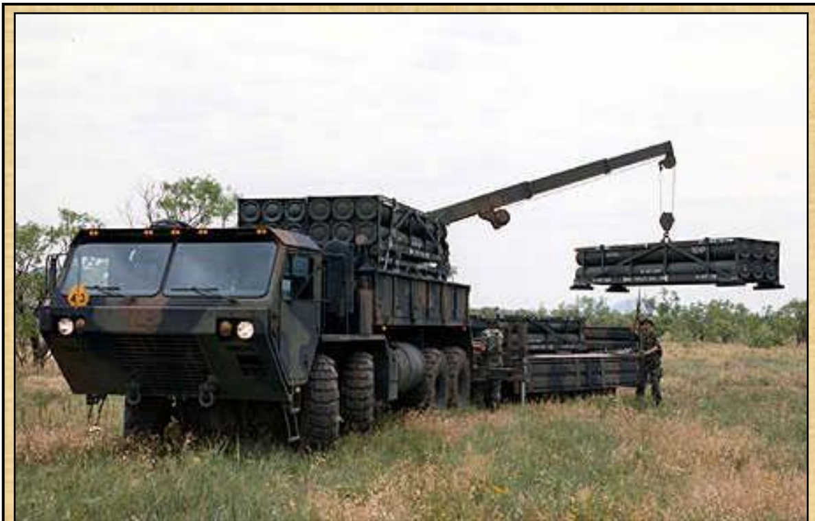
Figure 15-a An M-985 HEMTT (Heavy Expanded Mobility Tactical Truck) used for MLRS resupply operations. This one has a trailer.
