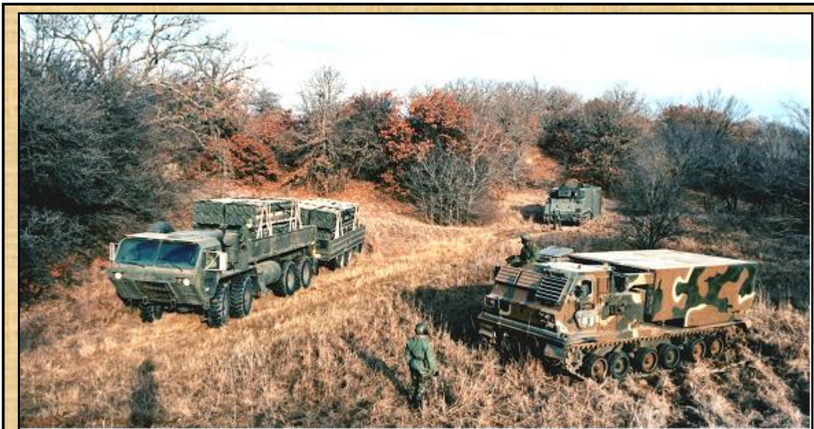
Figure 3-g MLRS as a Complete System: A view of a Multiple Launch Rocket System (MLRS) Self Propelled Launcher Loader (SPLL), right, a Heavy Expanded Mobility Tactical Truck (HEMTT) with an early trailer, and a tracked M-577 Armored Personnel Carrier (APC). It was these three vehicle components that when combined together created the “system” functionality in the term MLRS.
