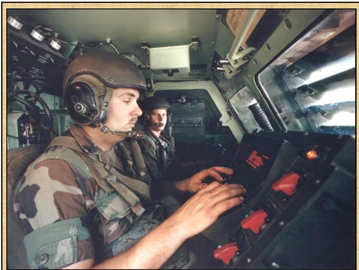
Figure 3-e Launcher Cab: An interior view of the launcher cab from the drover's side, showing the seating arraignment of the crew. On the right side (not show, here) sits the, Launcher Section Chief; usually a Staff Sergeant. In the middle sits the Gunner; a Sergeant who operates the Fire Control Panel. The driver is usually a junior enlisted soldier (seen here, behind the gunner).
