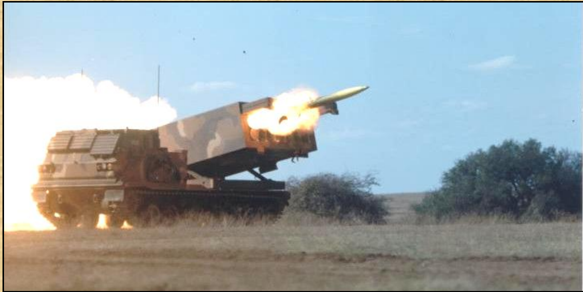
Figure 9-a Rocket Launch: A launch of an M26 rocket just moments after ignition. Within thirty-five feet of leaving the launch tub, a rocket will break the sound barrier. Note the size of the back blast plume behind the launcher.
