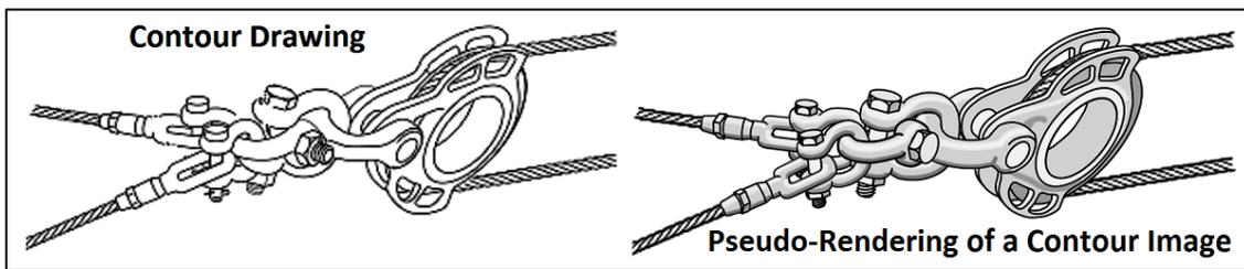
Figure 3-6. Rendering of a clevis and pulley system done with PowerPoint™
