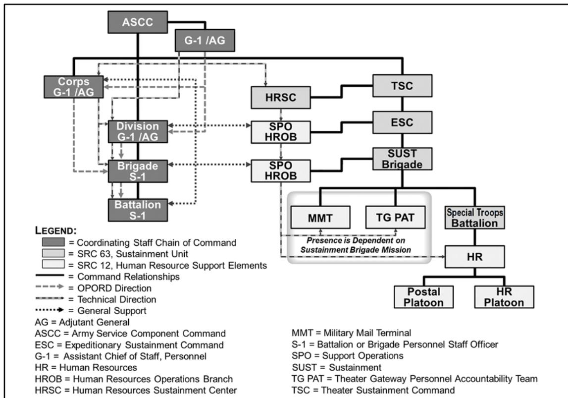
**Figure 3-20. A correctly developed (complicated) coordination chart**
